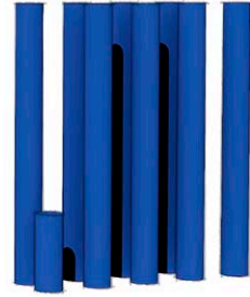
Traditional log wall. Logs can contain 65 kg/m 3 bound water at RH 75 %.
