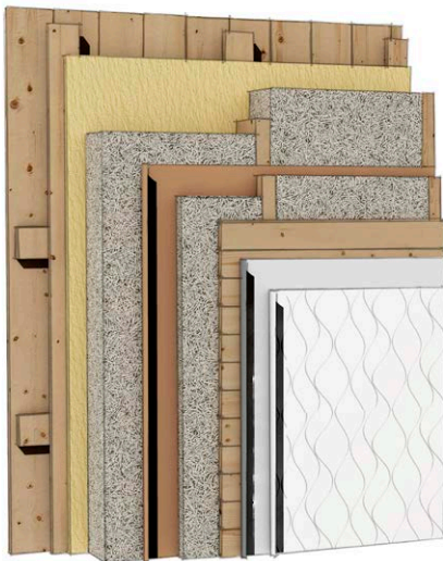
Contemporary cellulose fibre insulated wall. Cellulose fibre insulation (37 kg/m 3 ) can contain 4,1 kg/m 3 bound water at RH 75 %.
