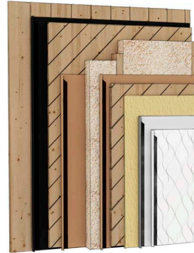
Traditional sawdust insulated wall. Sawdust can contain 19 kg/m 3 bound water at RH 75 %.
