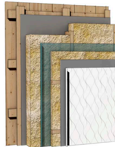
Contemporary mineral wool insulated wall. Mineral wool insulation can contain 0,36 kg/m 3 bound water at RH 75 %.
