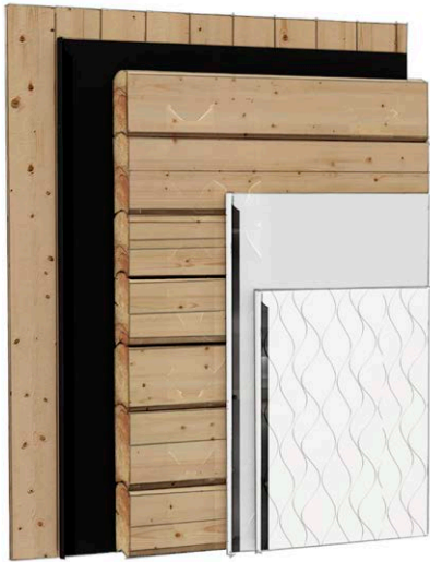
Traditional log wall. Logs can contain 65 kg/m 3 bound water at RH 75 %.
